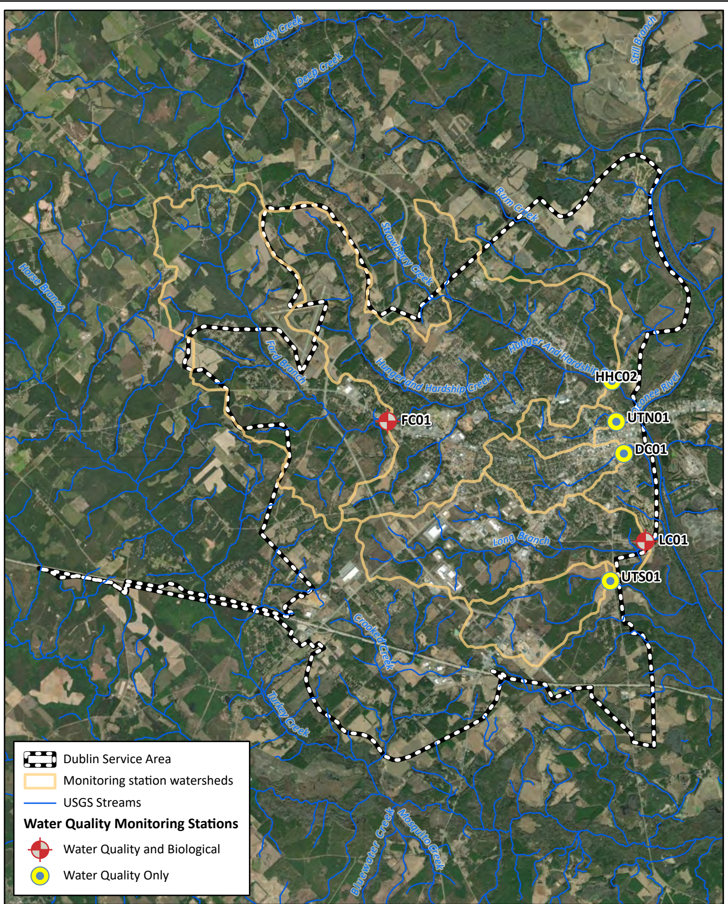
Figure 2. Long-term water quality monitoring stations for the Dublin Watershed Protection Plan.
