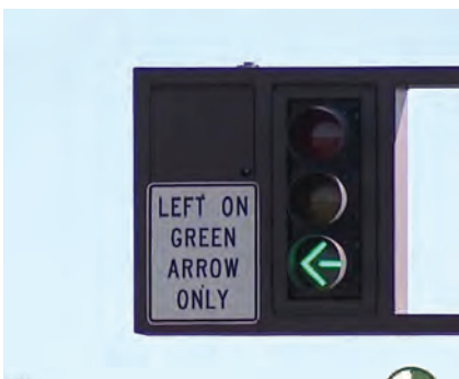
Protected Turn Lights
